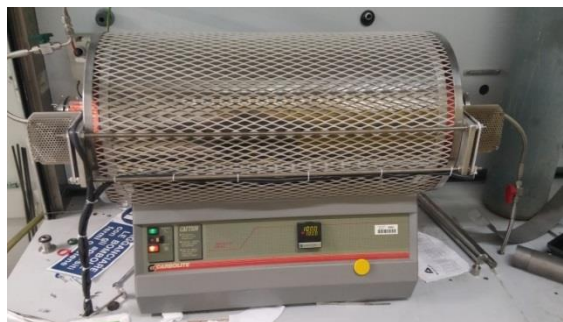
Figure 5. Quartz tube furnace adopted to sintered iron powder.
